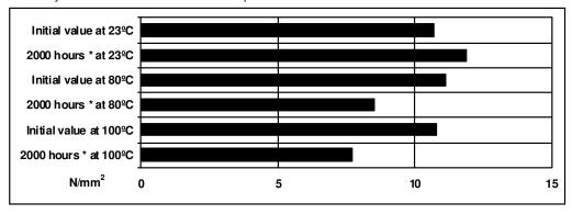
Immersion in water at specified temperature and tested at that temperature.
