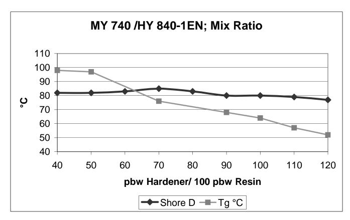
This casting resin system has low exothermic heat on cure. Volume of 250 g can be potted in typical parts (inlcuding PWB's), at room temperature. With bigger volumes or higher starting temperatures temperature might exceed 80 °C, cooling is recommended then.
